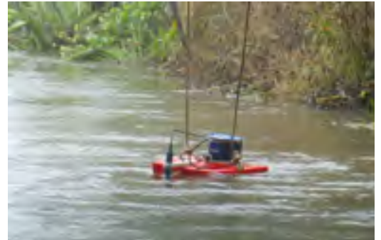
Photo (above): Flood Flow Monitor
